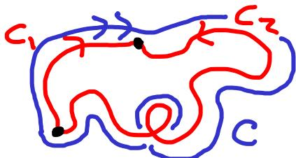
$$\begin{aligned} \int_{C_1} \mathbf{F} \cdot d\vec{r} &= \int_{C_2} \mathbf{F} \cdot d\vec{r} \iff \int_{C_1} \mathbf{F} \cdot d\vec{r} - \int_{C_2} \mathbf{F} \cdot d\vec{r} = 0 \quad (3) \\ &\iff \int_{C_1} \mathbf{F} \cdot d\vec{r} + \int_{\text{-}C_2} \mathbf{F} \cdot d\vec{r} = 0 \quad \text{Reverse orientation} \\ \text{glue paths together} &\quad \iff \int_C \mathbf{F} \cdot d\vec{r} = 0 \end{aligned}$$
