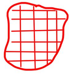
Then  $x$ -coord of center of mass is  $\bar{x} = \frac{1}{\text{total mass}} \iint_R x \rho(x, y) dA$
