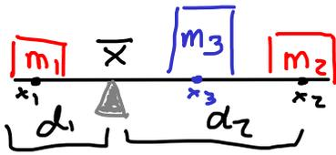
"center of mass"  $\bar{x}$  = place to put pivot (fulcrum) so that it's balanced.
