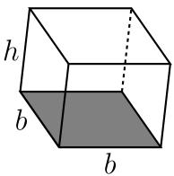
The volume of the box is  $V=b^2h$  and the surface area is  $S=4bh+b^2.$
